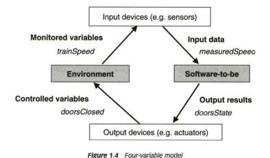
Generic architecture of a control system including embedded software [Lamsweerde]
